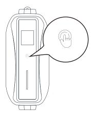
Adjust Current: Touch @ for 2 seconds until all the green LEDs flash. Then click to choose the current, selecting between 6A to 16A.
