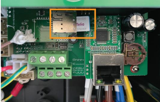
To establish the 4G connection please add a SIM card to the SIM card slot inside the charger. Please remove the front cover to reach the SIM card slot inside the charger. Before installing the SIM card, remove the PIN from the card.
