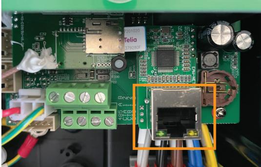
To establish the Ethernet LAN connection please insert one side of a network cable into the charger's RJ45 port and the other end to switch with outside network connectivity.
